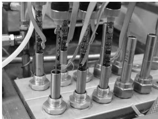
Fig 3: Laboratory set-up of differential pressure humidity generators
